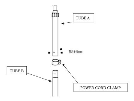
**Step 5:** Attach the HEATER HEAD to the top of TUBE A. Use two ST4\*12mm screws to secure the HEATER HEAD to TUBE A. Tighten until secure. Clip the power cord to the two POWER CORD CLAMPS to secure the power cord. The unit is now assembled.
